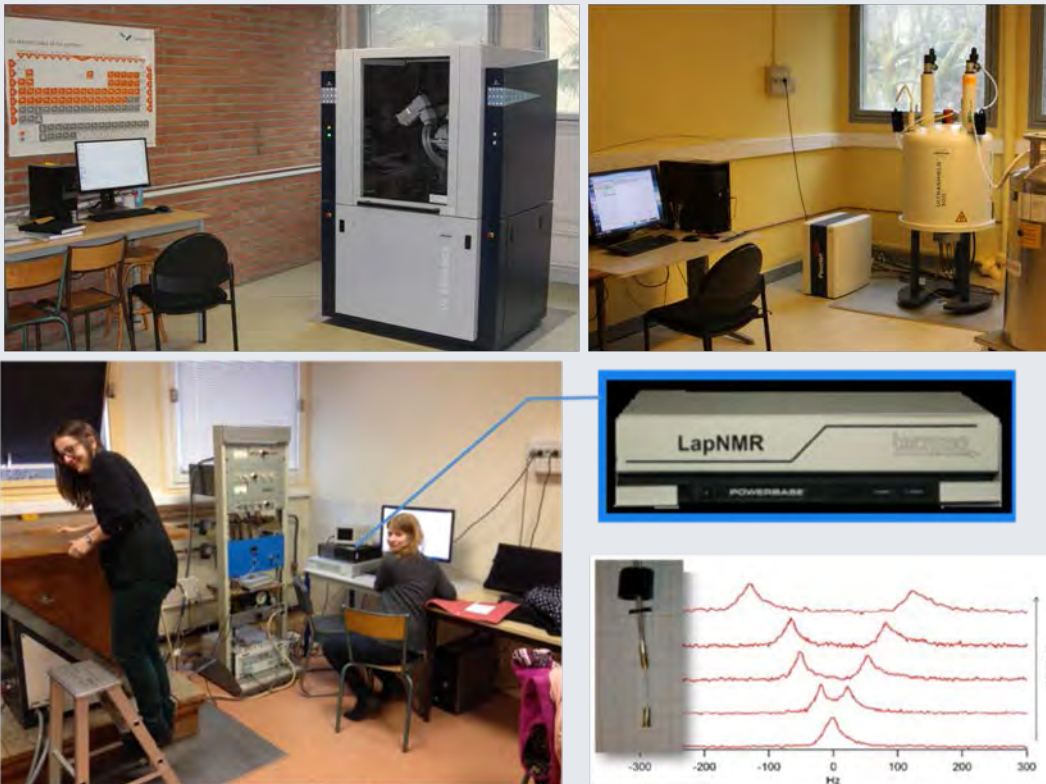
a few elements of the platform: NMR field, X-ray powder and central diffusion setup and generator, NMR spectrometer, data: a quadrupolar splitting of an NMR spectrum in deuterated rubber under strain
