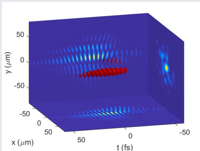
*3D reconstruction of the E-field amplitude of the UHI100 laser, measured at the focal point, by INSIGHT technique. On each side, the field projection on each coordinate is reported.*
