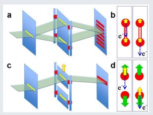
Schematic representation of the double slit gedanken experiment, with coupled (a) and decoupled (c) massive slits, and the schematics of the materialization of this thought experiment using a molecular photoionization experiment where the two slits are replaced by two coupled (b) and decoupled (d) oxygen atoms. The recoil momenta and the propagation directions of the dissociating atoms and electron are shown schematically by yellow, green and dashed blue arrows, respectively
